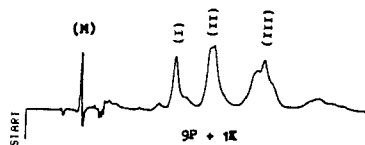
FIGURE - 2* HPLC chromatogram of synthetic admixture of 9 Petrol + 1 Kerosene (1% v/v in methanol).
